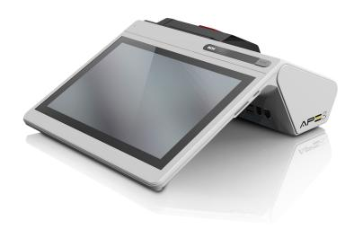
APE 3 is RCH's latest Android-powered solution. This all-in-one POS system features a compact and space-saving design, incorporating a high-quality thermal printer with 8 dots per mm resolution. The 10-inch touchscreen with In-Plane Switching (IPS) LCD technology provides operators with high-definition images, uniform brightness, and wide viewing angles.
